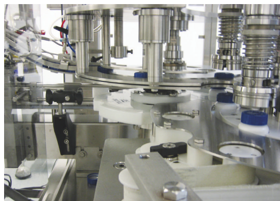
A new packaging line, top, combined existing equipment with a new vibratory-feed tablet counter and rotary capper. Bottom, the rotating cap-transfer starwheel picks the caps from the and the capping heads descend and pick up the caps for application to the bottles.
