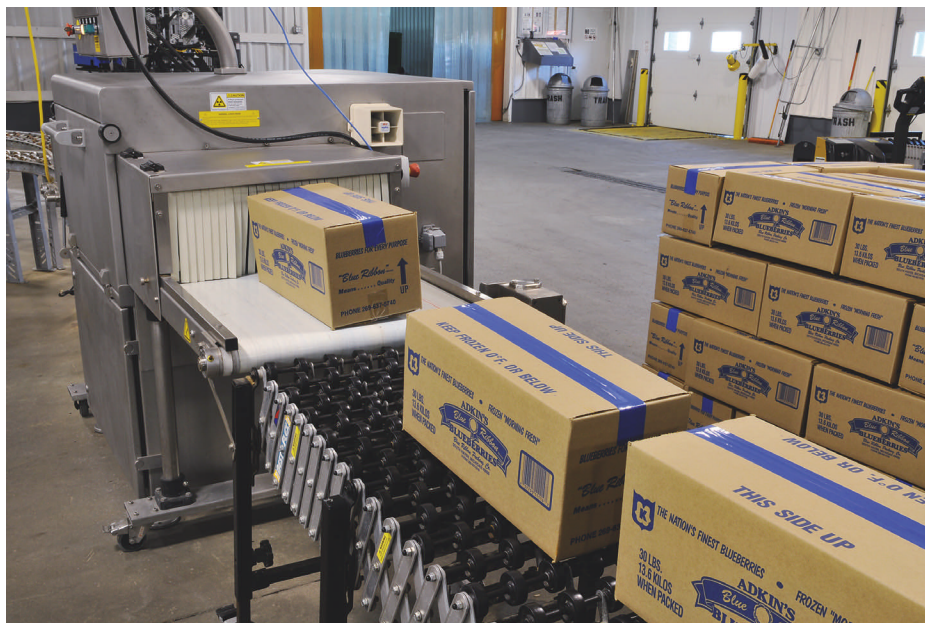
Cases of blueberries, above, exit the x-ray inspection system and are ready to be hand-palletized. The system detects metal, glass, stone and many other dense contaminants.
