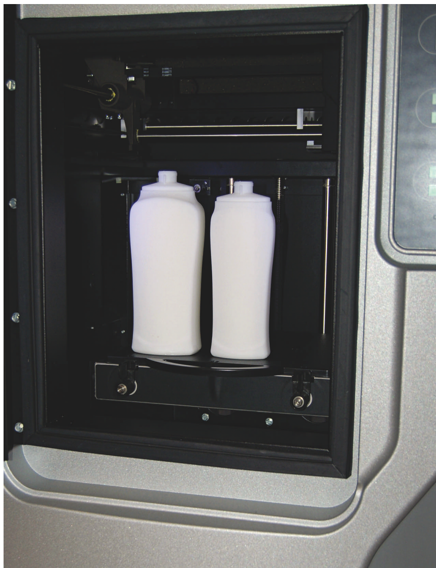
Silgan employs advanced design tools to create bottles that met the appearance requirements of Lornamead's project team. Fused deposition modeling is used for all custom and stock bottles. The FDM printers can create as many as 900 models a year.
