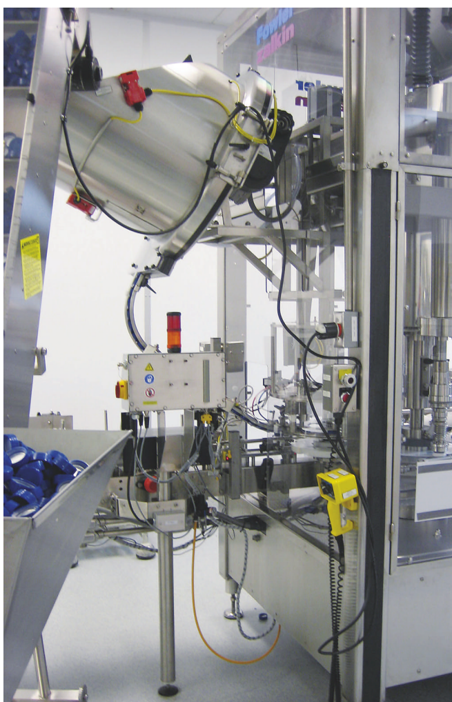
This six-head rotary capper is specifically designed for pharmaceutical applications. It is completely lube free and features quick, toolless changeover for cap and bottle handling parts.
